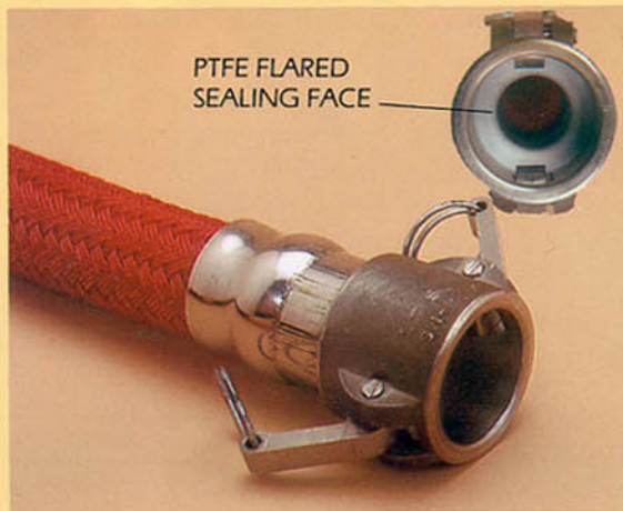
PTFE FLARED THROUGH ‘ARCLOCK’ CAM ARM COUPLING PTFE LINED UNDER SEAL. (Available with PTFE envelope gaskets rubber filled or fully encapsulated PTFE silicone filled seals)
